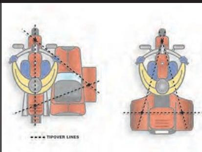
tip-over line. The reduced weight over the opposite side wheel can cause it to lift slightly.
